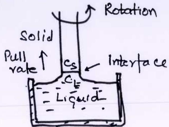
Crystals are pulled from the melt with certain Pull-rate and with spin rate of rotating Crystal.
