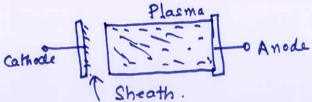
DC Discharge normally occurs at pressures of  $3 \times 10^{-2}$  torr and applied voltage in the range 100V to 300V.
