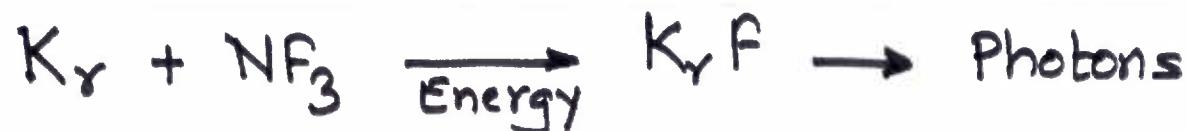
a) KrF -  $\lambda = 248 \text{ nm}$  (Used for Technologies  $0.13 \mu \text{ to } 0.25 \mu$ )
