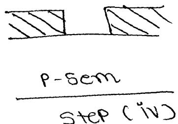
(iv) Using a mask and lithography technique window in Fox opened which has area of  $2\text{mm} \times 2\text{mm}$ . In this area we shall create gate-oxide.
