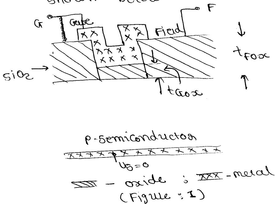
There are two capacitors observe here. One related to Gate oxide with thickness  $t_{\text{GOx}}$  and other one is due to Field oxide with thickness  $t_{\text{FOx}}$ .
