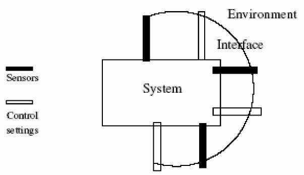
In a real-time system the events in the environment are detected by sensors and the responses to these events are generated in a timely manner. A RTOS ensures that control ættings (in response to an event) are achieved in real-time.
