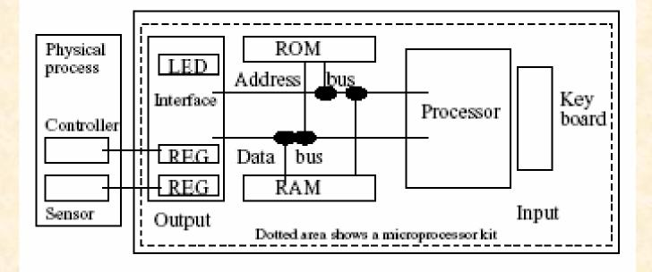
We can program the kit in machine language. The program can be directly stored in memory. On execution we observe output on LEDs. We also have some attached ROM. To simulate the operation of an embedded system input can be read from sensors and we can output to an interface to activate an actuator. We can use the timers and use these to periodically monitor a process. One can demonstrate the operation of an elevator control or a washing machine with these kits.
