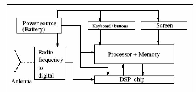
Power source is usually a lithium battery. It feeds the IO devices, the DSP chip and the processor and memory modules. There is also a RF to digital signal conversion module.
