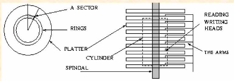
NOTE THAT THE RINGS ON THE DISC PLATTERS ON THE SPINDLE FORM A CYLINDER SINCE ALL HEADS ARE ON A PARTICULAR RING AT THE SAME TIME SO IT IS EASY TO ORGANISE INFORMATION ON A CYLINDER. THE INFORMATION IS STORED IN THE SECTORS THAT CAN BE IDENTIFIED ON THE RINGS. SECTORS ARE SEPARATED FROM EACH OTHER. ALL SECTORS CAN HOLD EQUAL AMOUNT OF INFORMATION
