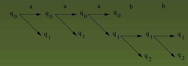
Definition A Nondeterministic Finite State Automaton (NFSA) is a 5-tuple  $M = (K, \Sigma, \delta, q_o, F)$ where  $K, \Sigma, \delta, q_0, F$  are as given for DFSA and  $\delta$ , the transition function is a mapping from  $K \times \Sigma$  into finite subsets of K. The mappings are of the form  $\delta(q, a) = \{p_1, \dots, p_r\}$ which means if the automaton is in state q and reads 'a' then it can go to any one of the states  $p_1, \dots, p_r$ .  $\delta$
