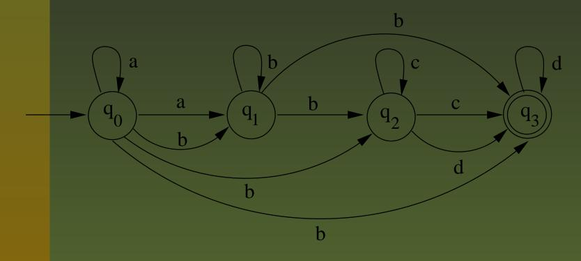
$\begin{aligned} \epsilon\text{-closure of } (q_0) &= \{q_0, q_1\} \\ \epsilon\text{-closure of } (q_1) &= \{q_1\} \\ \epsilon\text{-closure of } (q_2) &= \{q_2, q_3\} \\ \epsilon\text{-closure of } (q_3) &= \{q_3\} \\ \text{It is not difficult to see that the language accepted by} \\ \text{the above } NFSA &= \{a^n b^m c^p d^q / m \ge 1, n, p, q \ge 0\}. \end{aligned}$
