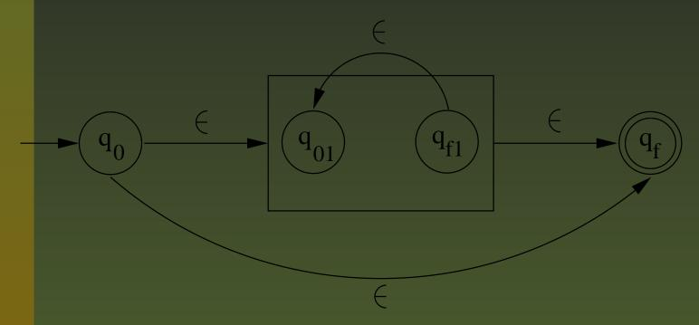
For this NFSA with  $\epsilon$ -moves  $q_0$  is the initial state and  $q_f$  is the final state. It can be seen that  $R_1^*$  contains strings of the form  $x_1, x_2, \ldots, x_k$ each  $x_i \in R_1$ . To accept
