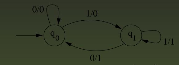
The input and output alphabet are  $\{0, 1\}$ . For the input 011010011, the output is 00110100 and machine is in state  $q_1$ . It can be seen that the first is 0 and afterwards, the output is the symbol read at the previous instant. It can also be noted that the machine goes to  $q_1$  after reading a 1 and goes to  $q_0$  after reading a 0.
