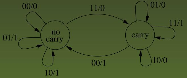
$p \rightarrow q$  denotes that when the adder is in state p and gets input  $x_1x_2$ , it goes to state q and outputs  $x_3$ . The input and output on a transition from p to q is denoted by i/o. It can be seen that suppose the two binary numbers to be added are 100101 and 100111.
