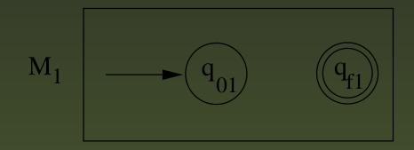
Without loss of generality we can assume that each such NFSA with  $\epsilon$ -moves has only one final state.  $R_2$  is similarly accepted by an NFSA  $M_2$  with  $\epsilon$ -transition.
