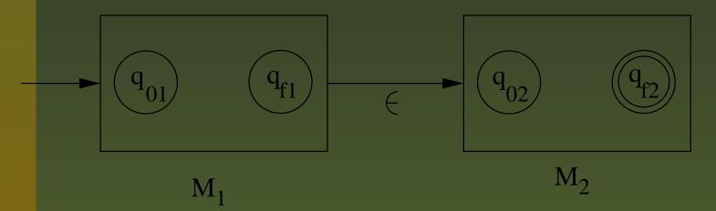
For this NFSA with  $\epsilon$ -moves  $q_{01}$  is the initial state and  $q_{f2}$  is the final state.  $R_1^* = R_1^0 \cup R_1^1 \cup R_1^2 \cup \cdots \cup R_1^k \cup \cdots$   $R_1^0 = \{\epsilon\}$  and  $R_1' = R_1$ . Introduction to Formal Languages, Automata and Computability - p.35/51
