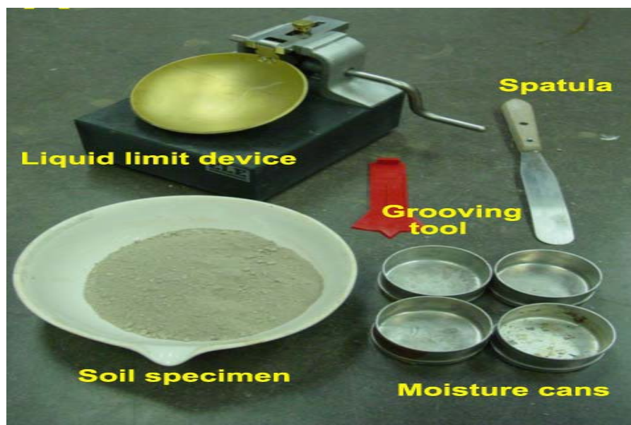
Figure 7.3: Casagrande apparatus used to find out liquid limit
