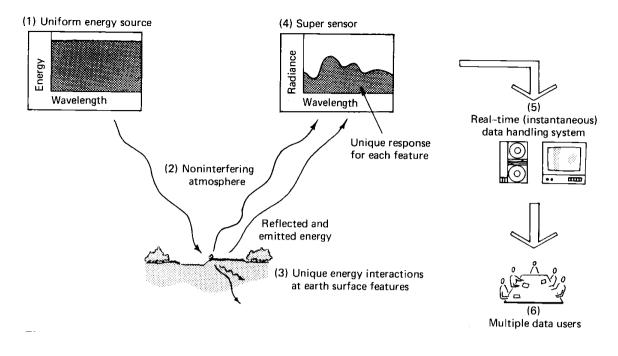
Fig. 7 Components of an ideal remote sensing system
