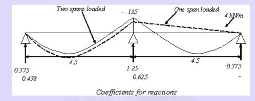
Maximum hogging moment =  $0.125 \times 29.3 \times 4.5 = 16.5 \text{ kNm}$ Maximum sagging moment =  $0.096 \times 29.3 \times 4.5 = 12.7 \text{ kNm}$
