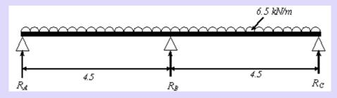
Factored load on each span = 6.5 x 4.5 = 29.3 kN
