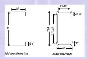
Thickness of steel (ignoring galvanizing), t = 2 - 0.04 = 1.96 mm Internal radius of the corners =  $1.5 \times 2 = 3$  mm
