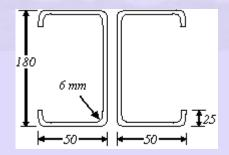
Try 180 x 50 x 25 x 4 mm Double section (placed back to back)
