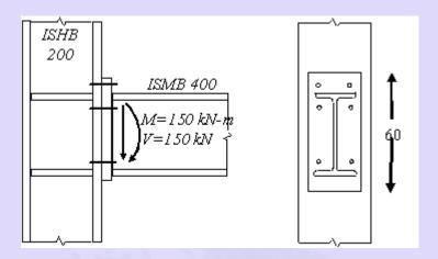
2) Thickness of end plate assuming 10 mm fillet weld to connect the beam with end plate, distance from center line of bolt to toe of fillet weld b = 60-10 = 50 mm; end plate width be = 180 mm effective width of end plate per bolt w = be/2 = 180/2 = 90 mm
