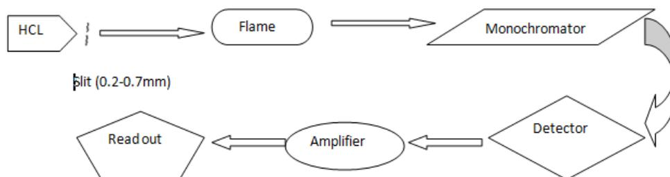
In AAS, the source of light is monochromatic and there is no need for entrance slit. However a slit of 0.2 or 0.7 nm is employed before the flame only to control the intensity of the incident radiation. . The light passes through the sample in the flame and then enters the monochromator. From the exit slit of the monochromator it falls on to the detector and the signal is amplified and readout.
