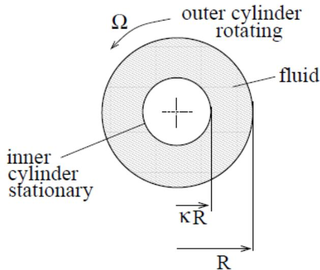
Figure 16: **Problem 18: Top view of the set-up with two concentric cylinders**
