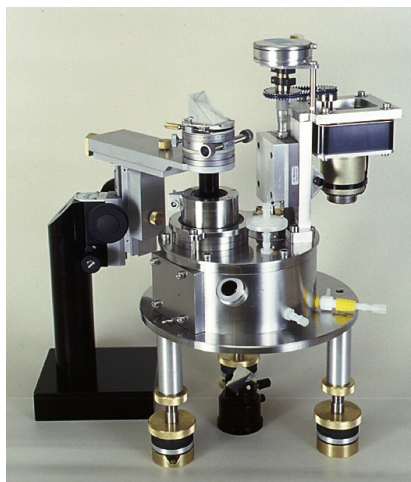
Fig. 3.2.2 Mark IV Surface Force Apparatus manufactured by The Australian National University (reproduced by permission from the Australian National University © 2009).
