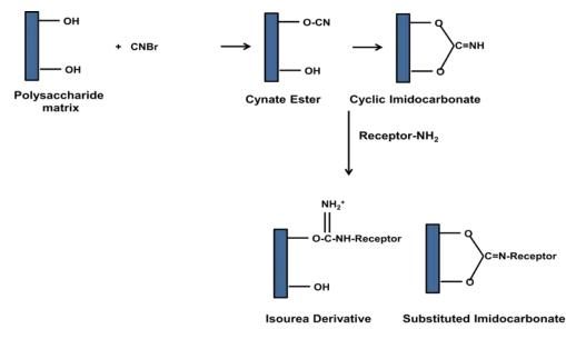
Figure 29.1: CNBr mediated coupling of receptor to the matrix.
