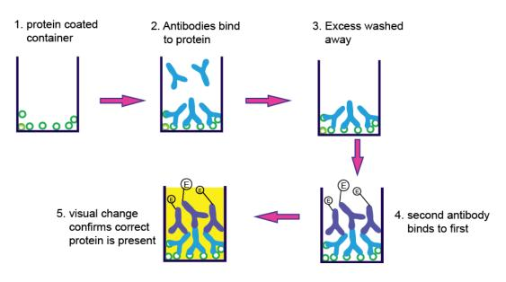
Figure 30.2: Different Steps in performing in-direct ELISA to measure antibody level in the serum.
