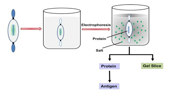
Figure 27.4: Electroelution using horizontal gel electrophoresis apparatus.
