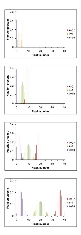
Figure 20.2 Separation of three components having different partition coefficients for the two phases
