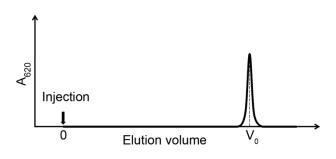
Figure 22.5: A chromatogram illustrating the void volume of a gel filtration column
