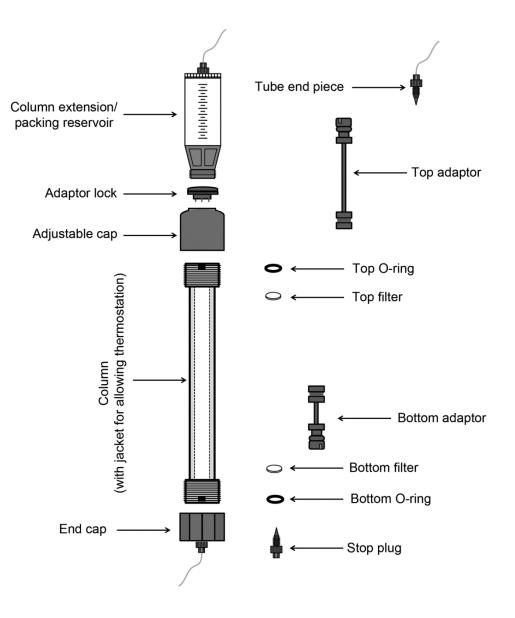
Figure 22.3 Column and its attachments
