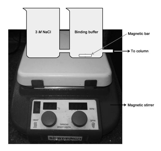
Figure 24.2: A gradient mixer kept on the magnetic stirrer
