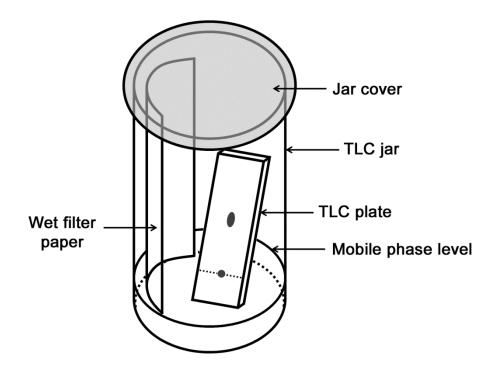
Figure 21.5: A thin layer chromatographic experiment set-up
