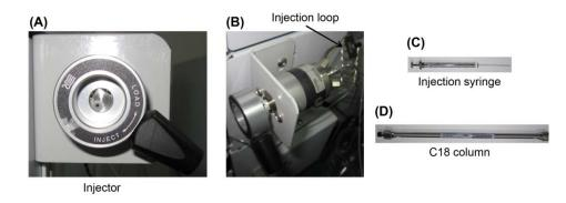
Figure 26.4: Injector in 'Inject' mode (panel A), an injection loop (panel B), an injection syringe (panel C), and a C18 column (panel D)
