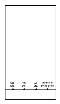
Figure 21.4: A thin layer chromatographic plate with spotted samples
