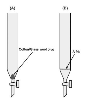
Figure 24.1: A column with cotton/glass wool plug (A); a fritted column (B)
