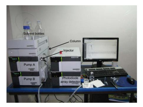
Figure 26.1: An HPLC instrument
