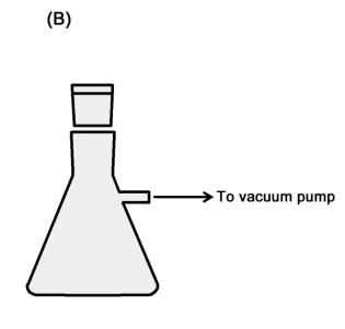
Figure 22.1: A buffer filtration unit (panel A) and an Erlenmeyer flask for degassing (panel B)
