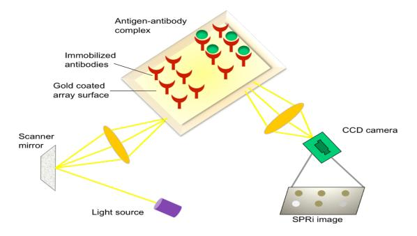
Fig 1. SPRi relies on measurement of changes in refractive index of the medium directly in contact with sensor surface.
