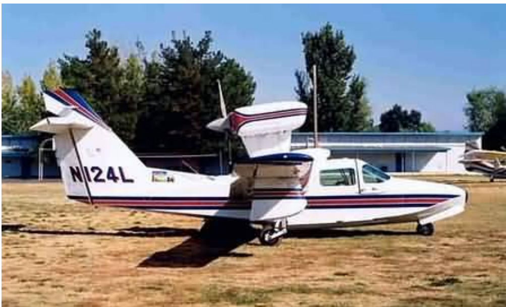
Fig.6.12 Image of an amphibian airplane with pod mounted engine and pusher propeller
