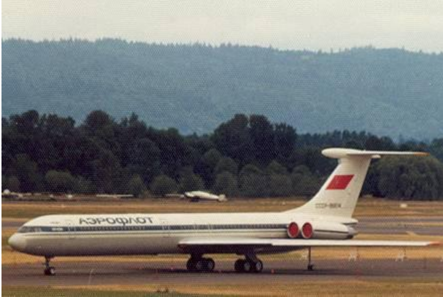
Fig.6.16 Image of a jet airplane with four engines mounted on pylons near the rear end of fuselage
