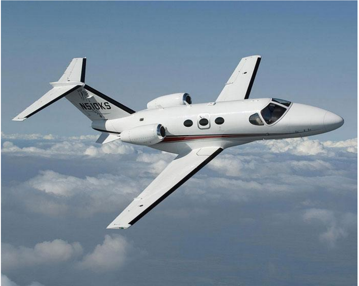
Fig.6.13 Image of a jet airplane with engines mounted on pylons near the rear end of fuselage (Adapted from aacjet.com)
