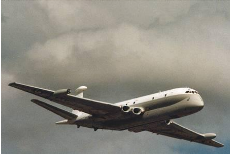
Fig.6.15 Image of a jet airplane with engines buried in wing root (Adapted from 1000aircraftphotos.com)
