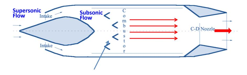
• The ramjet engine produces power by increasing the momentum of the working fluid by induction of energy by combustion of fuel, so that the momentum of the exhaust jet exceeds that of the incoming air, on a continuous basis.
