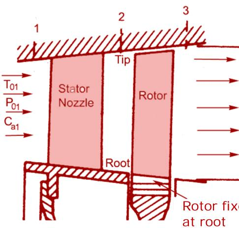
• Flow comes from the combustor with high internal energy  $(T_{01}, P_{01}, C_{a1})$ , and is made to go through the <u>stator</u> - where a large part of its internal energy is converted to kinetic energy.
