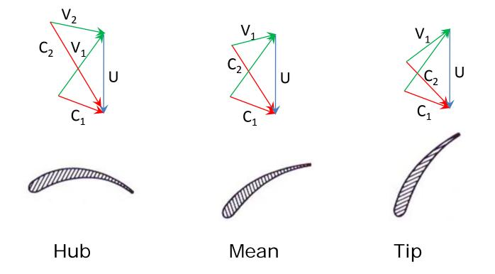
Free vortex velocity diagrams at the hub, mean and tip sections
