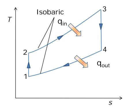
$T_1 = 27^{\circ}C = 300 \text{ K}$  $P_1 = 100 \, kPa$  $r_p = 6.25$  $T_3 = 800^{\circ}C = 1073 K$
