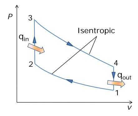
$T_1 = 35^{\circ}C = 308 \text{ K}$   $P_1 = 0.1 \text{ Mpa}$   $T_3 = 1100^{\circ}C = 1373 \text{ K}$  $r = v_1/v_2 = 7$
