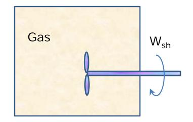
Raising of a weight by a rotating shaft does not generate entropy, and so energy is not degraded during this process (if we assume frictional effects can be neglected). The work done on a gas increases the entropy of the gas, and thus energy is degraded during this process.
